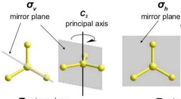
$\sigma_v$  mirror plane contains the  $C_3$  axis
