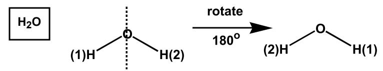
Line in molecular plane, bisecting HOH angle is a rotation axis, giving indistinguishable configuration on rotation by 180°.
